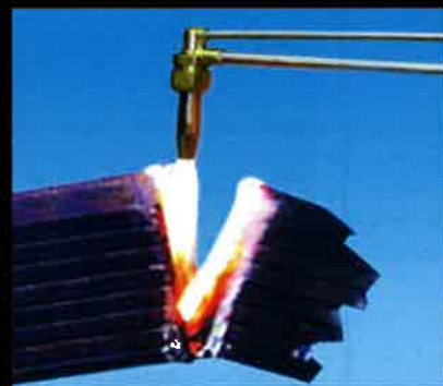
Cutting 8 layers steel sheet
